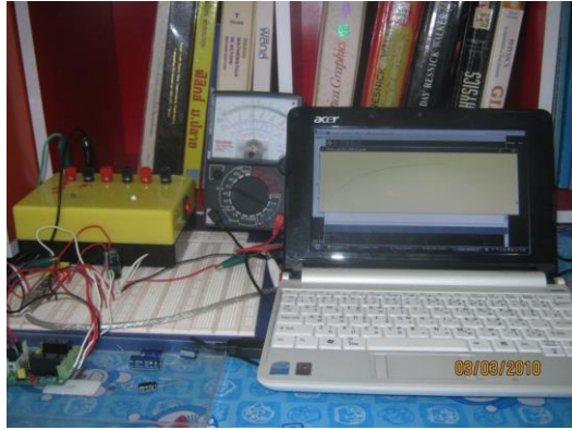
Fig. 4 : Computer interface experiment of charging and discharging of a capacitor in real time physics teaching.
